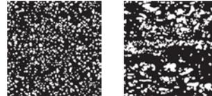
The uniform distribution of carbides in the powder-metallurgical structure compared to conventional tool steels with big carbides and carbide clusters.
